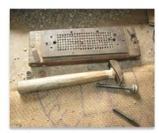
Plate2. Hammer for cutting the punch card
