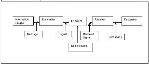
Figure 1. Communication as a mechanistic system
